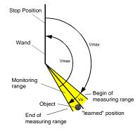
Fig. 3-2: "Start" cycle with CW travel
