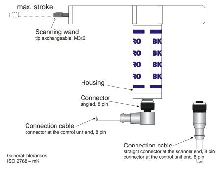
Fig. 2-24: Scanner TK9LIN50
