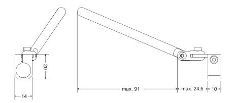
Fig. 2-23: Dimensions Mounting Bracket / Holding arm
