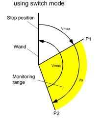
Fig. 3-8: "Start" cycle with scanning in both directions
