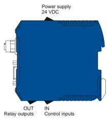
Fig. 2-2: BK MIKRO9 Control Unit – Connection positions
