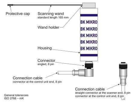
Fig. 2-19: Scanner TK94A / TK94RL
