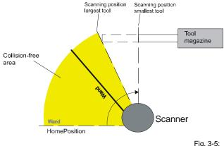
Fig. 3-5: Time-optimized scanning – "Collision-free area"
