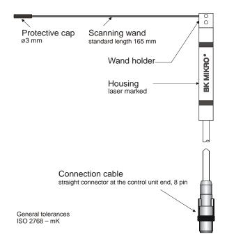
Fig. 2-21: Scanner TK96A / TK96RL
