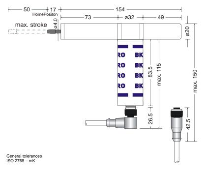
Fig. 4-9: Mechanical Dimensions – Scanner TK9LIN50
