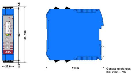
Fig. 4-2: Mechanical Dimensions – I/O Expansion Module
