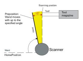
Fig. 3-4: Time-optimized scanning – Preposition
