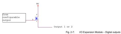
The outputs are high-side-switches, which means that, they act like normal switches: Either they actively switch 24V (max. 0,5 A) on the output or the output is unused.
