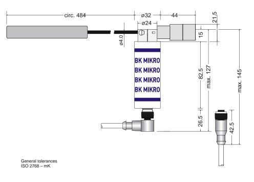
Fig. 4-5: Mechanical Dimensions – Scanner TK91A
