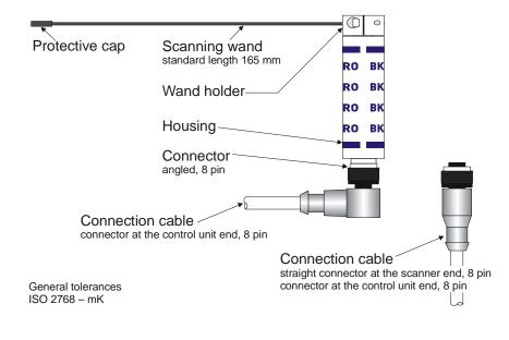
Fig. 2-13: Scanner TK7A / TK7RL
