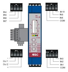
Fig. 2-5: I/O Expansion Module – Connections
