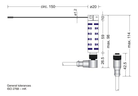
Fig. 4-3: Mechanical Dimensions – Scanner TK7A / TK7RL
