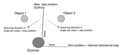
Fig. 3-3: Scanning CW / CCW
