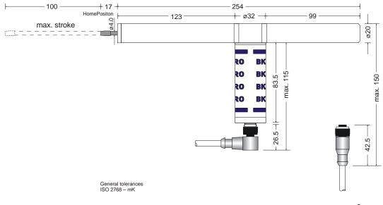
Fig. 4-11: Mechanical Dimensions – Scanner TK9LIN100
