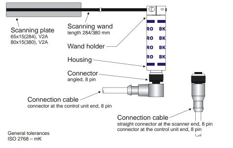
Fig. 2-14: Scanner TK8A
