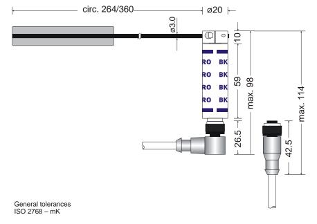
Fig. 4-4: Mechanical Dimensions – Scanner TK8A
