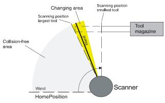
Fig. 3-6: Time-optimized scanning – "Time frame"
