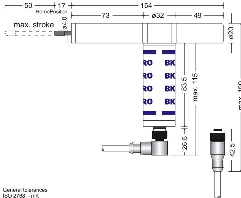
Fig. 4-9: Mechanical Dimensions – Scanner TK9LIN50
