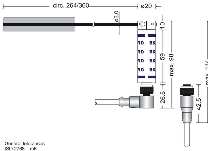
Fig. 4-4: Mechanical Dimensions – Scanner TK8A
