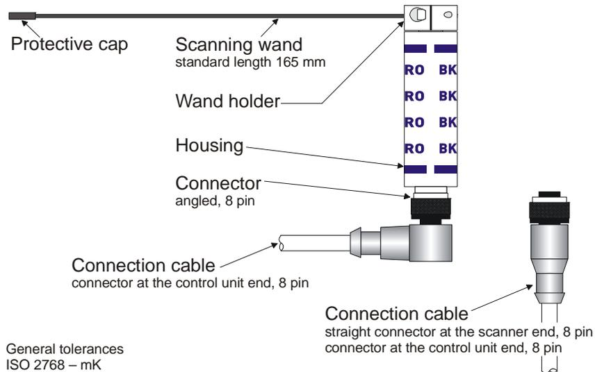
Fig. 2-13: Scanner TK7A / TK7RL
