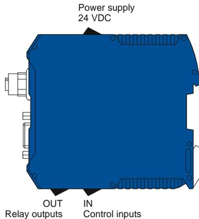
Fig. 2-2: BK MIKRO9 Control Unit – Connection positions
