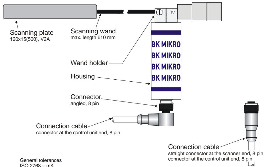
Fig. 2-15: Scanner TK91A with 3 balance weights
