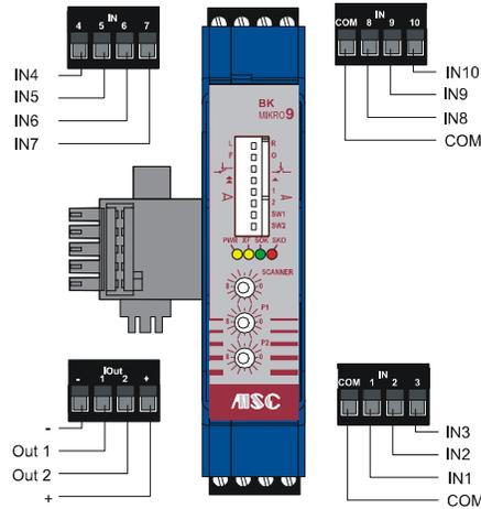
Fig. 2-5: I/O Expansion Module – Connections
