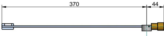
Fig. 2-17: Dimensions in mm with 2 different balance weights
