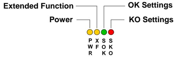
Fig. 2-8: I/O Expansion Module – Light-emitting diodes
