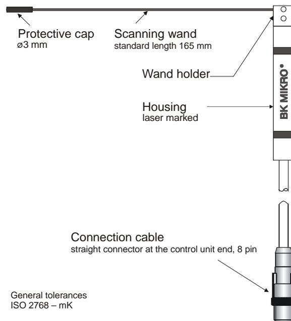
Fig. 2-21: Scanner TK96A / TK96RL
