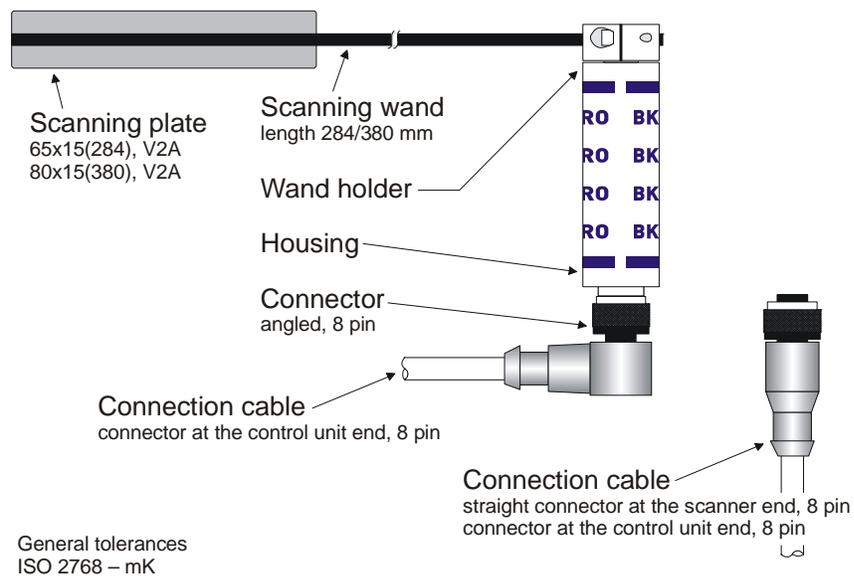
Fig. 2-14: Scanner TK8A
