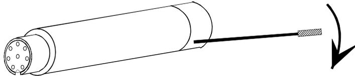
Fig. 2-11: Definition of the rotation direction
