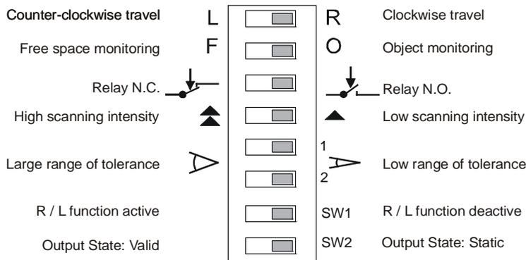
Fig. 2-10: I/O Expansion Module – Toggle switches
