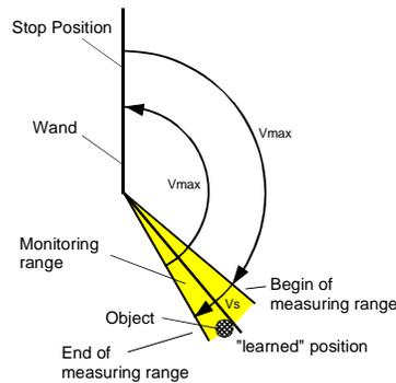
Fig. 3-2: "Start" cycle with CW travel
