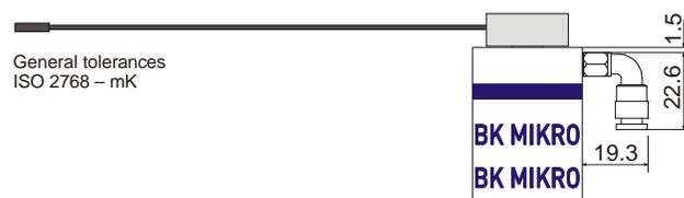
Fig. 4-7: Mechanical Dimensions – Option Air barrier light adapter
