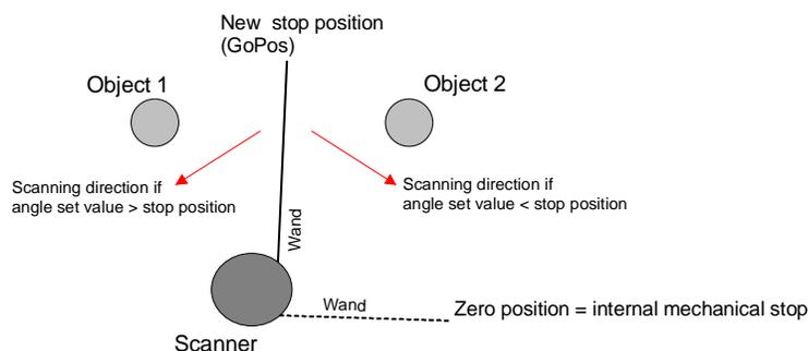
Fig. 3-3: Scanning CW / CCW
