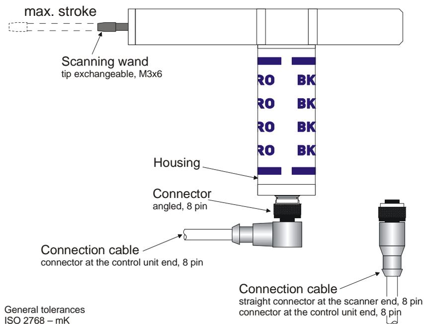
Fig. 2-24: Scanner TK9LIN50
