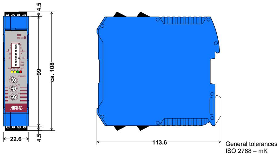
Fig. 4-2: Mechanical Dimensions – I/O Expansion Module
