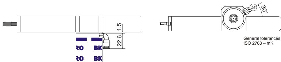
Fig. 4-10: Mechanical Dimensions – Option compressed air connection
