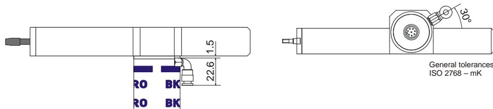
Fig. 4-12: Mechanical Dimensions – Option compressed air connection
