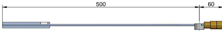
Fig. 2-16: Dimensions in mm with 3 balance weights
