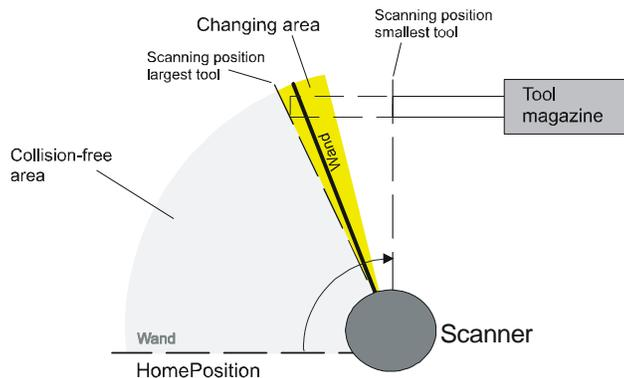
Fig. 3-6: Time-optimized scanning – "Time frame"
