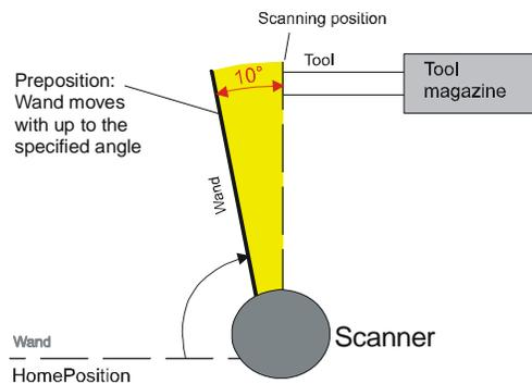
Fig. 3-4: Time-optimized scanning – Preposition
