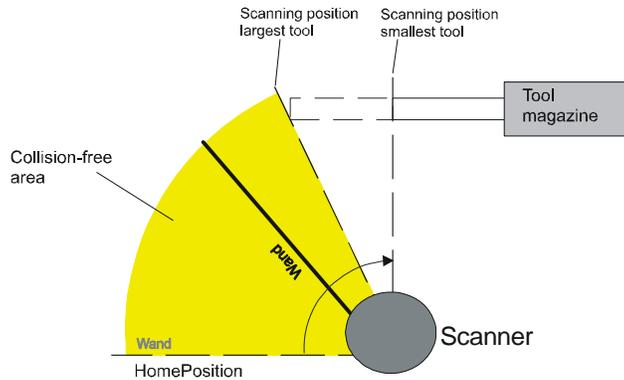
Fig. 3-5: Time-optimized scanning – "Collision-free area"
