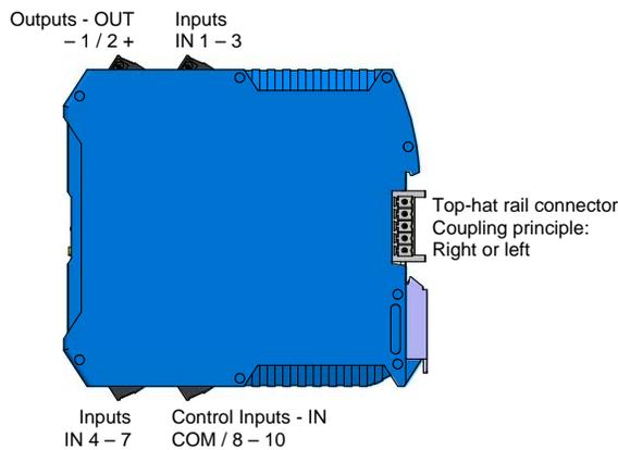
Fig. 2-6: I/O Expansion Module – Connections positions
