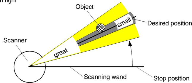
Fig. 2-12: Range of tolerance
