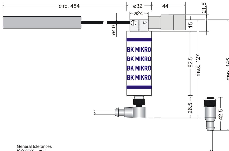
Fig. 4-5: Mechanical Dimensions – Scanner TK91A
