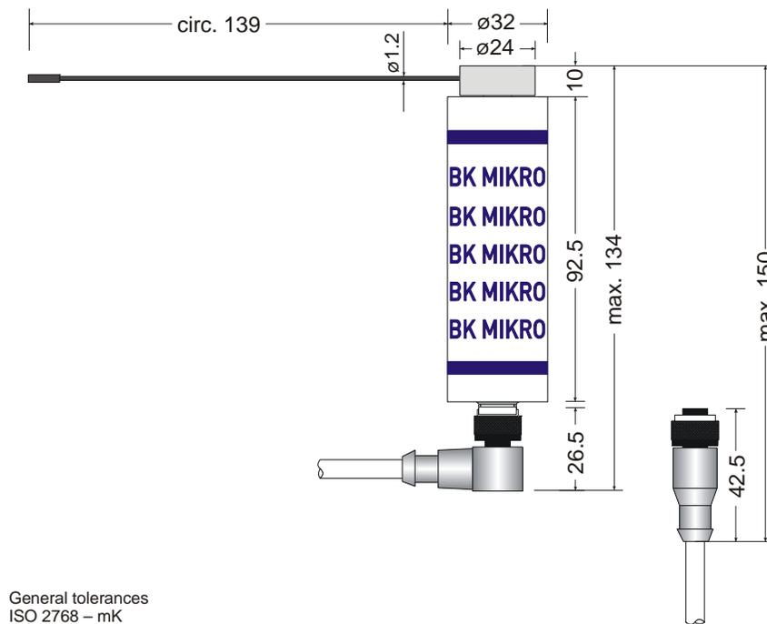
Fig. 4-6: Mechanical Dimensions – Scanner TK94A
