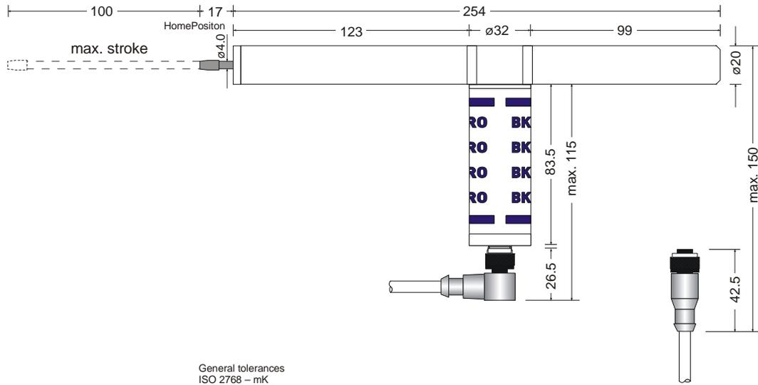
Fig. 4-11: Mechanical Dimensions – Scanner TK9LIN100
