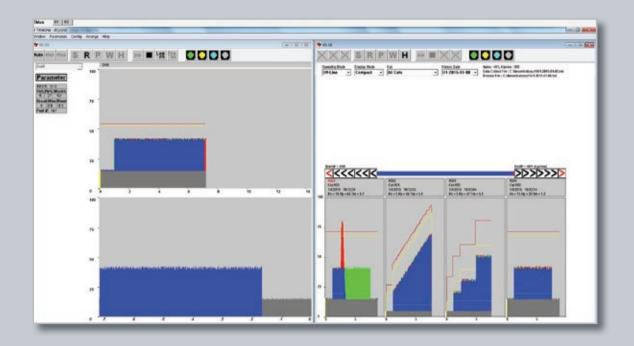
The Windows based TECHNA-CHECK<sup>®</sup> TTMON program is a powerful tool monitoring software for use on PC systems. The software is required for use with the PCI & USB systems.
