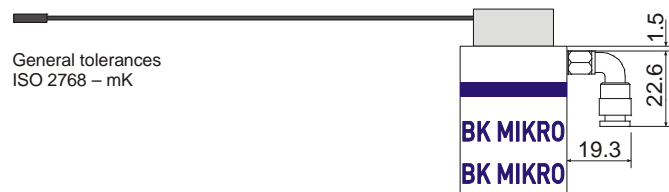
Fig. 4-7: Mechanical Dimensions – Option Air barrier light adapter
