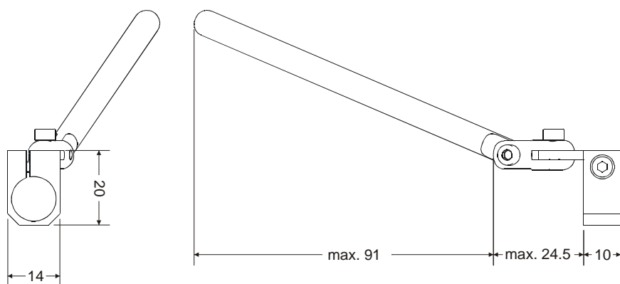
Fig. 2-23: Dimensions Mounting Bracket / Holding arm
